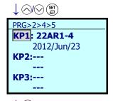
5. Use the  $\bigcirc$  /  $\bigcirc$  keys to select the location, KP1-KP3, to store the data to be confirmed, and confirm the destination with the (st) key.
