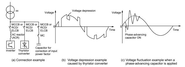
• Use an ACR when the interphase voltage unbalance ratio of the inverter power supply exceeds 2%.
