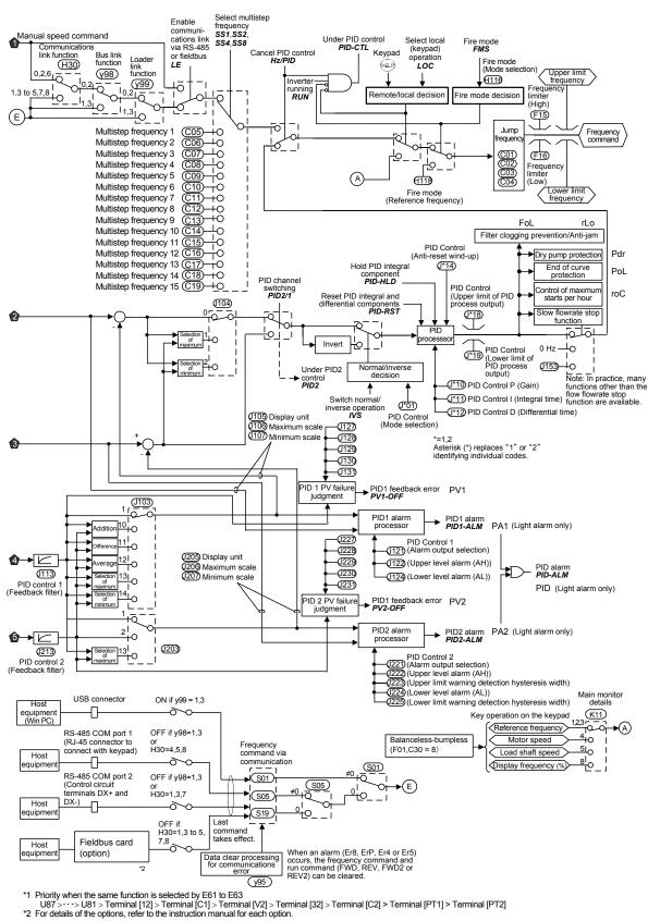
Figure 7.4 (2) PID Process Control Block
