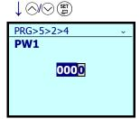
5. Use the  $\bigcirc$  /  $\bigcirc$  keys to select any four numerical digits, and confirm with the  $\stackrel{\text{(st)}}{=}$  key.
