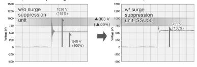
Motor/inverter capacity: 75 kW Wiring length: 100 m Running status: No-load
