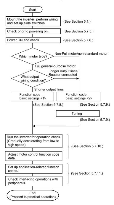
Figure 5.16 Test Run Procedure
