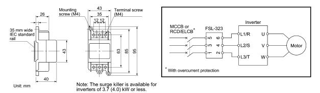
Figure 4.3 Dimensions of Surge Killer and Connection Example
