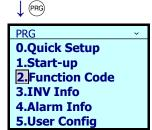
2. Use the ⊘/ ⊗ keys to select [2. Function Code], and confirm with the (♣) key.
