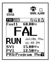
Fig. 9.1 Light alarm display example
