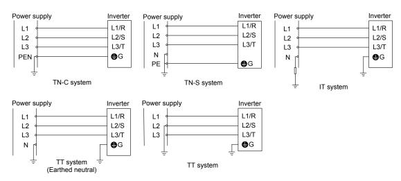
200V type inverters can be used at IT or TT system.
