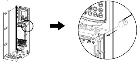
(3) Hook the battery harness over the boss and then fully insert the connector into connector CN11 on the control printed circuit board.
