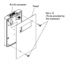
Figure 5.9 Mounting the Keypad
