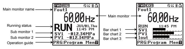
The display type can be selected easily in Programming mode as follows. |PRG > 1(Start-up) > 4(Disp Setting) > 1(Disp Mode)
