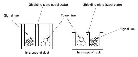
Figure A.7 Separate Wiring
