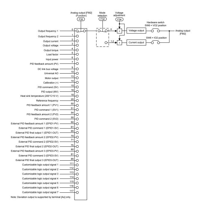
Figure 7.7 Terminal [FM2] Output Selector
