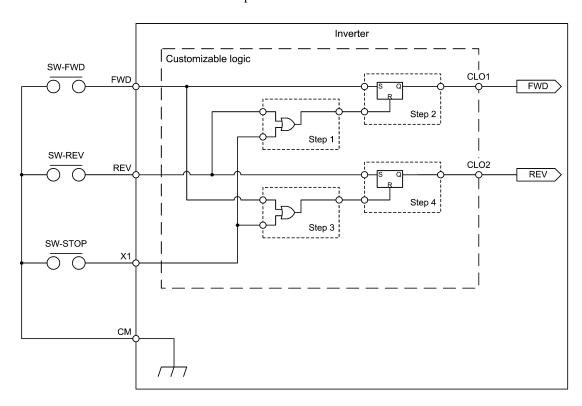
To configure the above customizable logic, set function codes as listed below. The "Type of timer" and "Time setting" require no modification unless otherwise specified.
