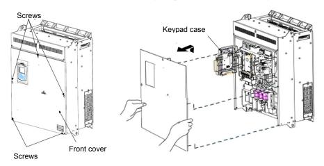
Figure 5.3 Removing the Front Cover and the Wiring Plate (FRN110AR1S-4□)
