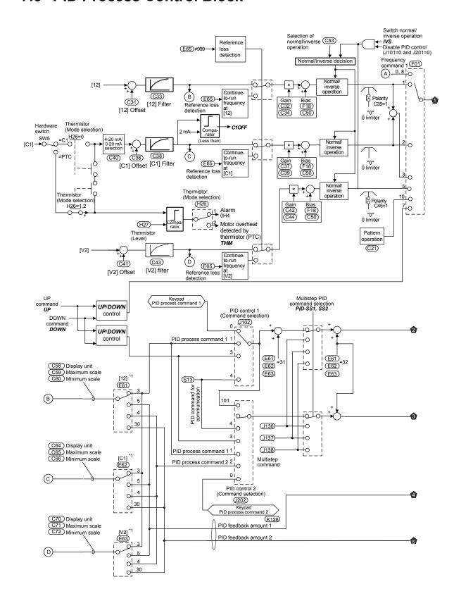
Figure 7.4 (1) PID Process Control Block
