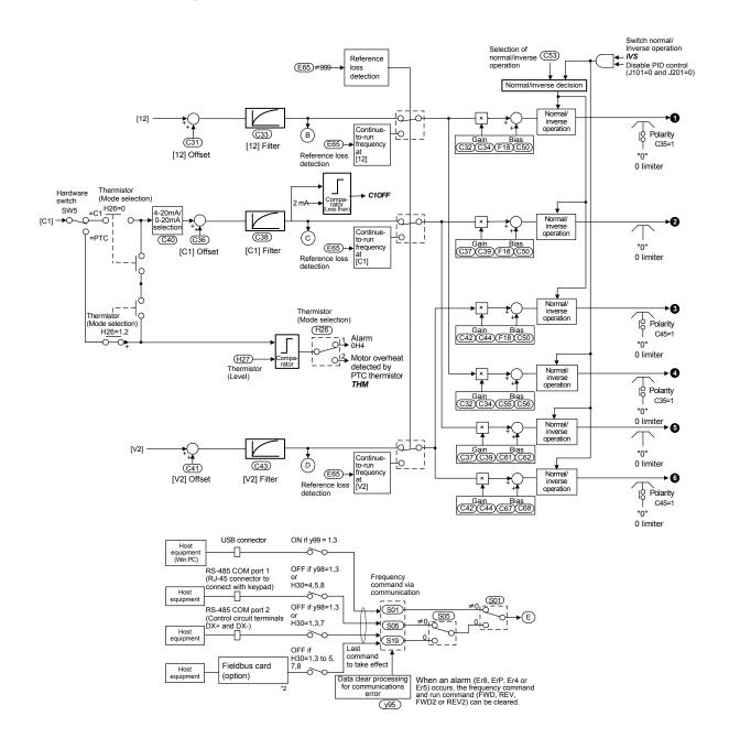
Figure 7.1 (1) Frequency Command Block
