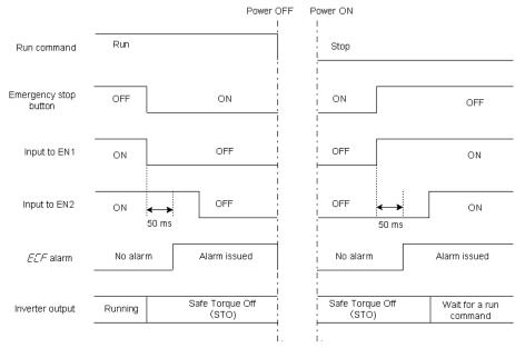
Figure 11.8  $\it ECF$  Alarm (Caused by Logic Discrepancy) and Inverter Output State
