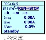
4. On the mode selection screen, use the ⟨⟨⟩/⟩ keys to move the Cursor, and select "RUN→STOP". Confirm with the (♣) key.
