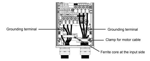
Figure 11.1 Wiring to Main Circuit Terminals
