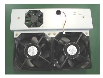
(5) Remove the fans from the fan unit using the procedure given below.
