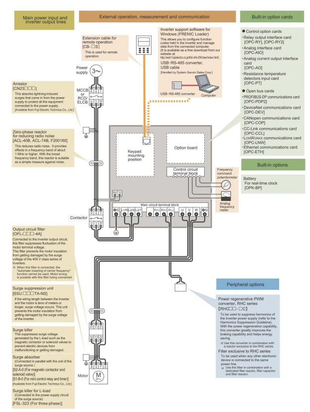
Figure 4.1 Configuration Example
