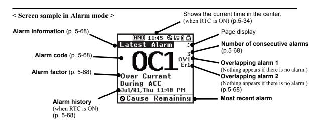
Figure 5.12 Screen Samples In Running and Alarm Modes
