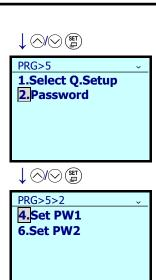
3. Use the  $\bigcirc / \bigcirc$  keys to select [2. Password], and confirm with the  $\stackrel{\text{(st)}}{=}$  key.
