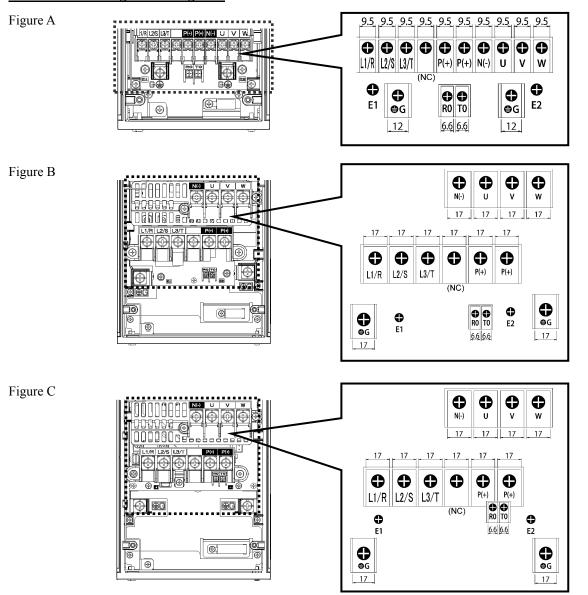
(NC): No connection (Do not make wiring.)
