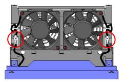
(4) Remove four screws and cut the cable ties. Rotate the fans to the direction shown with arrows and remove the fans from fan case.
