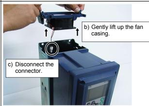
(3) Remove the cooling fan from its casing. See d).
