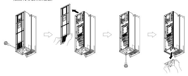
Figure 5.2 Removing the Front Cover and the Wiring Plate (FRN37AR1M-4□)
