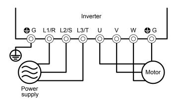
Figure 5.17 Connection of Main Circuit Terminals
