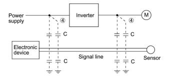
Figure A.5 Electrostatic Induced Noise
