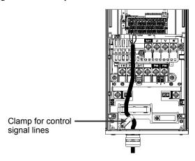
Figure 11.2 Wiring to Control Circuit Terminals
