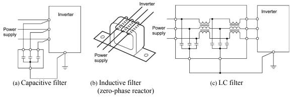
Figure A.10 Various Filters and their Connection
