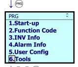
2. Use the ⊘/ ⊗ keys to select [6. Tools], and confirm with the (\$\sqrt{\text{gr}}\text{ key}.
