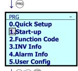
2. Use the ⊘/ ⊗ keys to select [1. Start-up], and confirm with the (♣) key.
