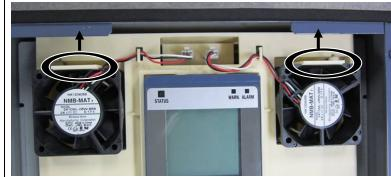
(3) Mount the internal fans in the reverse order of removal.
