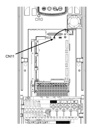
Figure 4.14 Battery Loaded (200 V class series inverters of 3.7 kW or below and 400 V ones of 7.5 kW or below)
