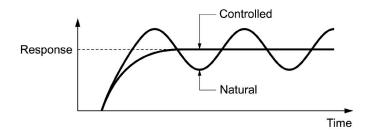
■ Feedback filter (PID control 1: J113 / PID control 2: J213)
