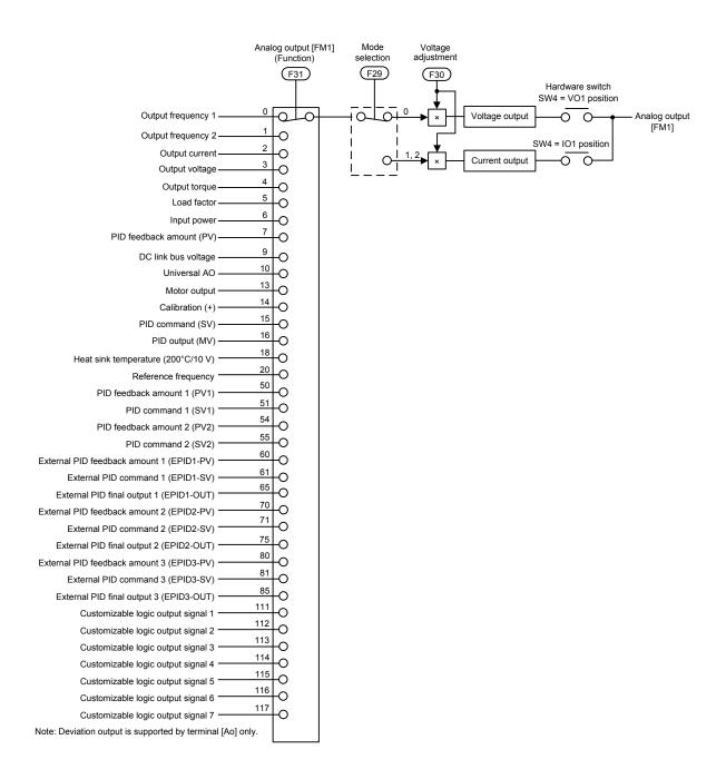
Figure 7.6 Terminal [FM1] Output Selector
