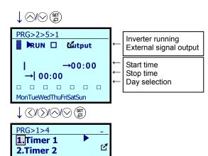
5. Use the () / () keys to shift the cursor, and use the () / () keys to input the check mark, time and day.
