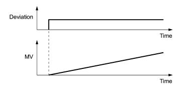
■ D differential time (External PID control 1: J512, External PID control 2: J612, External PID control 3: J662)
