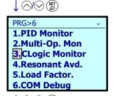
3. Use the \( \backslash / \overline{\overline{\overline{\text{keys}}}} \) keys to select [3. CLOGIC Monitor], and confirm with the \( \begin{array}{c} \setminus \text{key}. \end{array} \) key.
