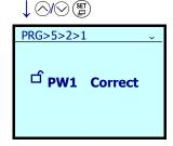
6. The set password is verified, and function code revision is enabled (password protection off).
