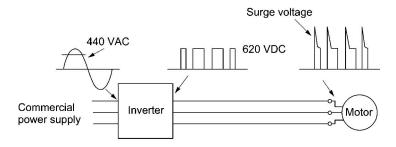
Figure B.1 Voltage Waveform of Individual Portions
