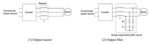
Figure B.3 Method to Suppress Surge Voltage
