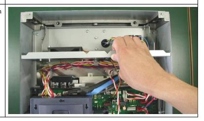
(4) The photo given at the right shows the fan unit removed.
