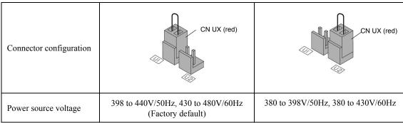
Note The allowable voltage fluctuation range is +10% to -15%.
