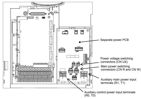
Figure 5.4-1 Location of Switching Connectors (200 V class series inverters of 22 to 45 kW and 400 V ones of 45 to 90 kW)
