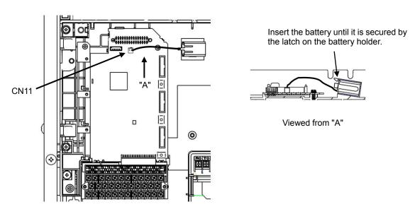
Figure 4.16 Battery Loaded (110 kW or above)
