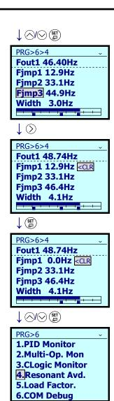
7. Using the key to move the cursor to Fjmp3 and pressing the key at the next point of resonance sets resonance prevention point 3 (Fjmp3).
