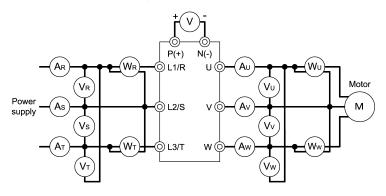
Figure 10.1 Connection of Meters
