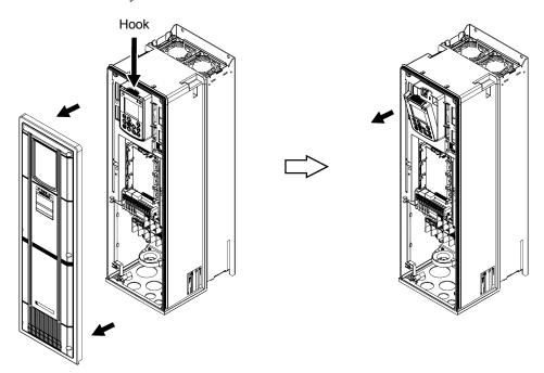
Figure 5.7 Removing the Keypad
