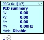
PID (final) information SV: Command value PV: Feedback value Err: Deviation MV: Manipulated value Mode: PID mode
