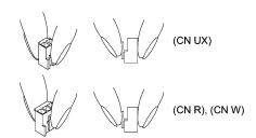
Figure 5.4-4 Removing/Inserting the Jumpers
