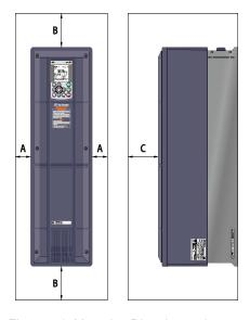
Figure 5.1 Mounting Direction and Required Clearances
