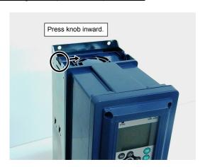
Remove the cooling fan (with case).
